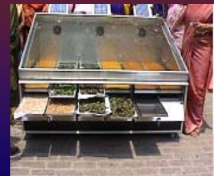
PV operated community Solar Drying system
