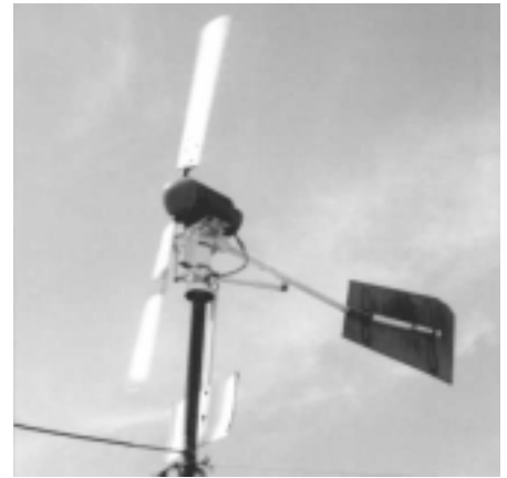
A typical small system (100-W wind generator) provides electricity for lighting, TV, and radio (130 kWh/a.).
