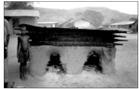
Efficient kiln to smoke fish. Note the 4 trays and the iron sheet covering them.
