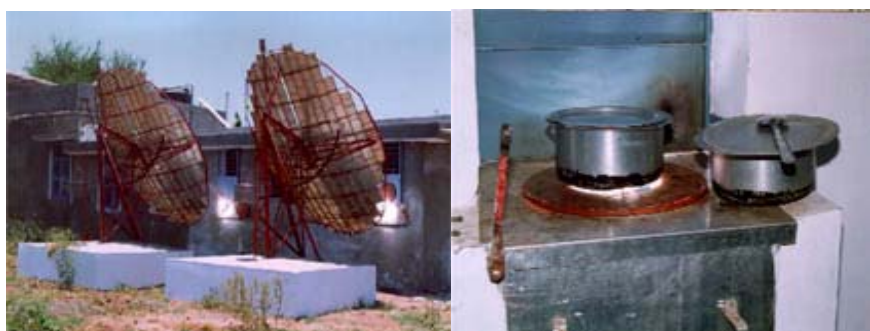
Scheffler concentrating cookers with a view of kitchen
