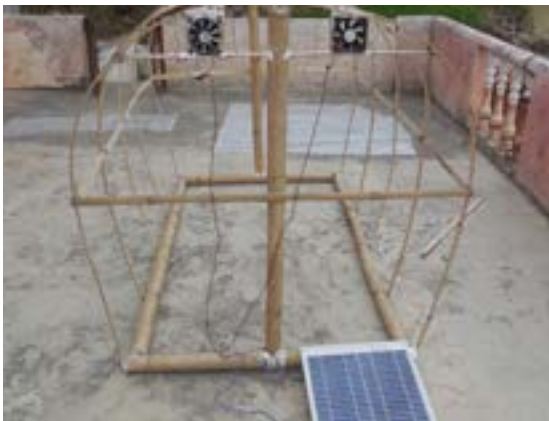
Solar poly tunnel dryer; drying vegetables; and construction of the top part from bamboo.
