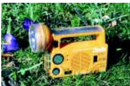
The PV powered radio and lamp
