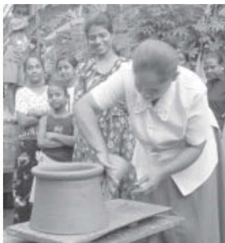
A step in the production of the Anagi two-pot clay stove (top), the finished stove (top-right), and the stove integrated in a kitchen under a chimney-hood (right)
