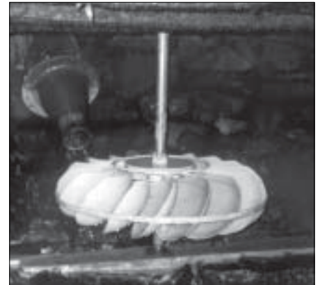
The penstock and kit runner of an improved water mill.
