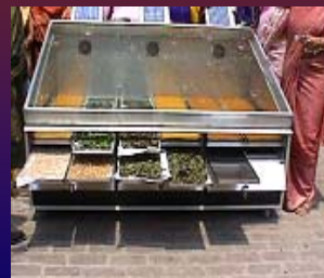
PV operated community Solar Drying system
