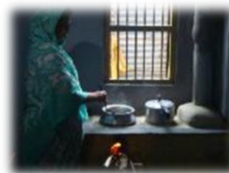
Improved cookstove (single Burner, with chimney)
