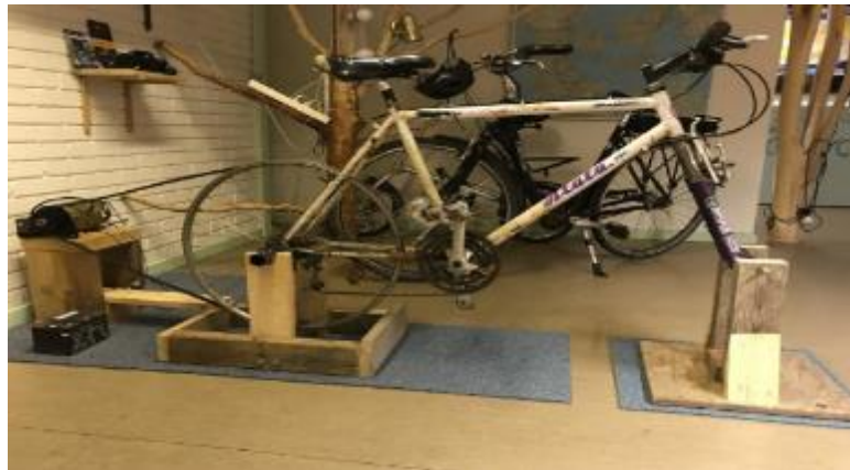
Static bike for charging power banks
