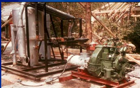
Wood gas electricity generation
